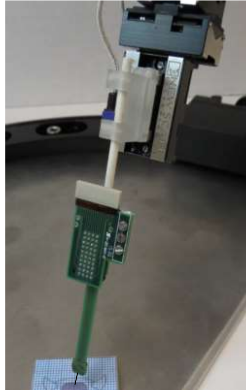
Figure 6: MPM Probe Mount-2, mounted on the insertion (Z) axis of an M3-LS motorized three-axis manipulator, with the NeuroNexus A32 Silicon Probe and OM32 Adapter installed.
