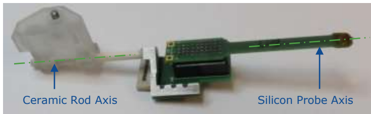
Figure 5: Using the MPM Probe Mount-2, the axes of the silicon probe and the ceramic rod are parallel and concentric.
