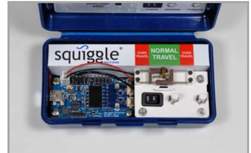
Figure 5: SQL-RV-1.8 Developer's Kits are battery-operated, ready-to-use kits that include a motor, controller, position sensor (for closed-loop kits) and New Scale Pathway™ software.
