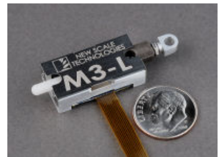
M3-L linear module with closed-loop controls integrated in a 17.5 x 13 x 7.5 mm package
