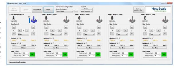
A single PC widow displays up to five probe controls at once (and up to eight with horizontal scrolling).
