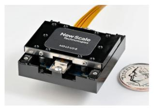
**The M3-LS-U2-8 Linear Smart Stage** is an ultra-compact positioning stage with submicrometer resolution and absolute encoding. *All electronics are built into the stage* for simple system integration. This model features power-off hold, high speed, and is cost-effective for high volume manufacturing.
