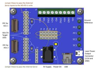
Jumper these to pass the Internal Servo Generator to the M3-RS-U units
