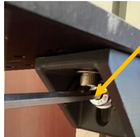
Loosen upper angle bracket screws
