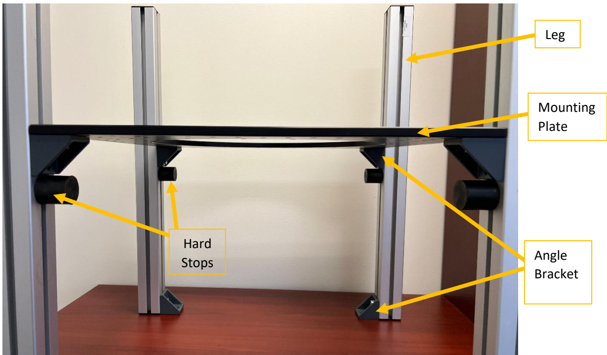
MPM-Platform assembled with (4) MPM-Ring-72 Deg sections installed
