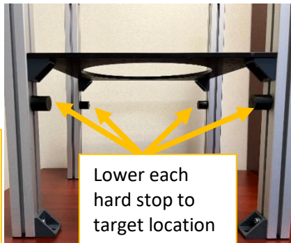
Measure to the top of the rubber hard stop
