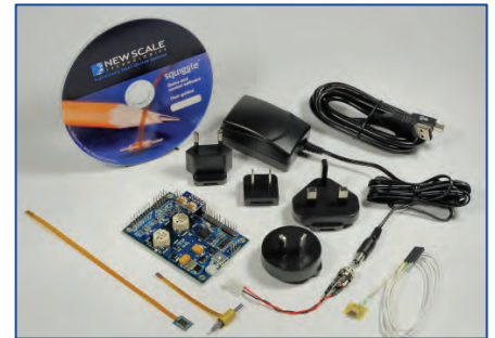
SQL-3.4 Evaluation Packs available for rapid implementation into your prototype designs. Open loop or closed loop (w/ TRACKER NSE-5310) systems available.
