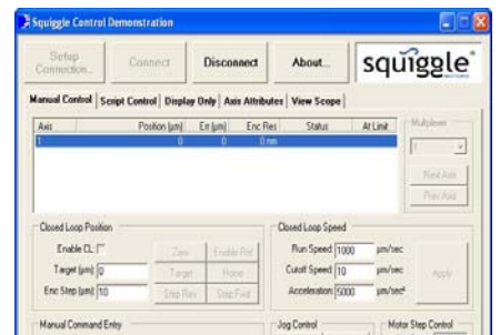
New Scale Pathway™ software provides point-and-click PC control, Active X command library and an intuitive scripting interface.
