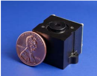
M3 micro-mechatronics modules – fully integrated motion systems including actuator, position sensor, guide mechanism, drive and control electronics and software.
