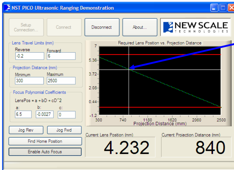
Figure 4: PC demonstration program showing projector auto focus in progress
