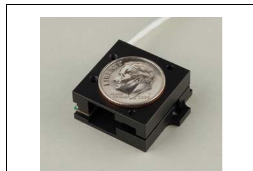
Figure 3 - This smaller closed-loop stage has 10 microns resolution and measures 25x25x10 mm. It uses a Hall Effect sensor and an SQL series SQUIGGLE motor.
